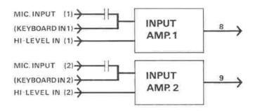
These amplifiers are used when a signal or control voltage from another instrument is to be put in to the SYNTHI. Before connecting anything other than another EMS Device, you should make sure that the signals are electrically suitable. For a description of the procedure you should adopt when making connections, see the section CONNECTING THE SYNTHI above; for details of signal levels, see the SPECIFICATIONS section (page 19).
