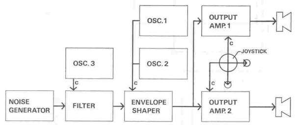
The source is the Noise Generator, and the signal is processed by the Filter and Envelope Shaper before being taken to both Output Amplifiers. Oscillator 3 controls the Filter, and Oscillators 1 and 2 control the Envelope Shaper; both Output Amplifiers are controlled by the joystick, which provides two Control Voltages. The effect of these controls will be described in the next section, here we are only concerned with the connections. Now consider this diagram:
