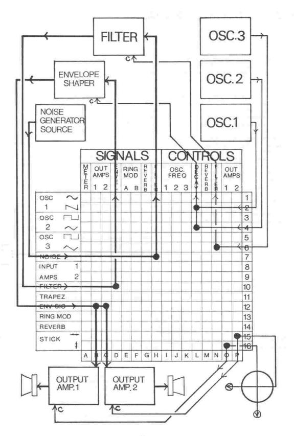
Although the boxes have been moved around somewhat the connections are the same. The important addition is that we have incorporated the patchboard, and marked the pins with blobs on the signal routes. Considering the signal only, this patch was achieved along the following lines:
