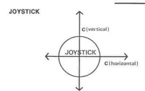
The Joystick is a very useful device, enabling you to alter two control voltages simultaneously. These voltages appear on the patchboard at rows 15 and 16. Although the mounting is round, the Joystick moves in a square whose corners correspond to the extremes of each voltage. The voltage swing for a particular movement of the joystick can be controlled by the RANGE controls beside it.
