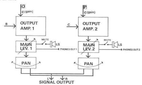
These Amplifiers are used at the end of a chain of devices to send the signal to the internal loudspeakers, headphones, or to an external taperecorder or amplifying system. Their inputs are rows B and C on the patchboard and all patches should have a pin in one or both of these rows.
